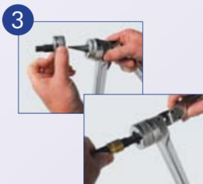
3 Expand the pipe using the PSC Expanding Tool making sure the jointing sleeve is well away from the area of pipe to be expanded. Expand the pipe twice to make a good expansion of the pipe end.
