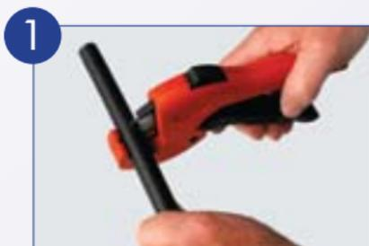
1 Cut the pipe to be joined cleanly and squarely using PSC PE-X Pipe Cutters.
