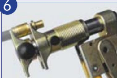
Draw the sleeve towards the fitting by closing the jaws of the Compression Tool until the sleeve reaches the shoulder of the fitting.
