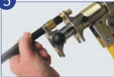
Slide the jointing sleeve towards the fitting. Position the jointing sleeve and the fitting squarely within the jaws of the PSC Compression Tool.
